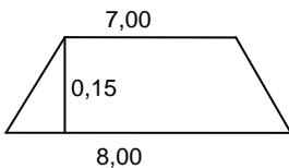
$$S = \left( \frac{7,00\text{m} + 8,00\text{m}}{2} \right) \times 0,15\text{m} = 1,125\text{m}^2 \approx 1,13\text{m}^2$$
